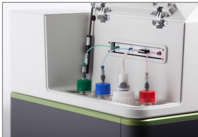
Figure 7.2: The reagent bottles and waste bottle inside their compartment. Bottle labels should face the front of the instrument (not the side).
