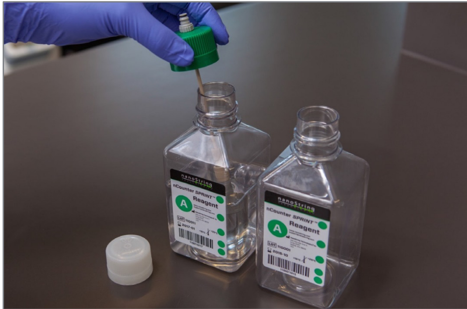
Figure 7.6: Switch caps between reagent bottles.
